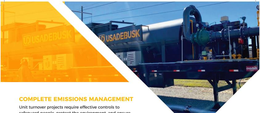
Unit turnover projects require effective controls to safeguard people, protect the environment, and ensure regulatory compliance. USA DeBusk offers specialized processes that collect and treat flammable and hazardous gases and vapors using thermal oxidation and combustion, degassing vapor recovery, and carbon adsorption.
